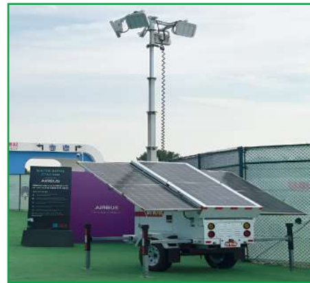
Solar-powered Lighting Towers
