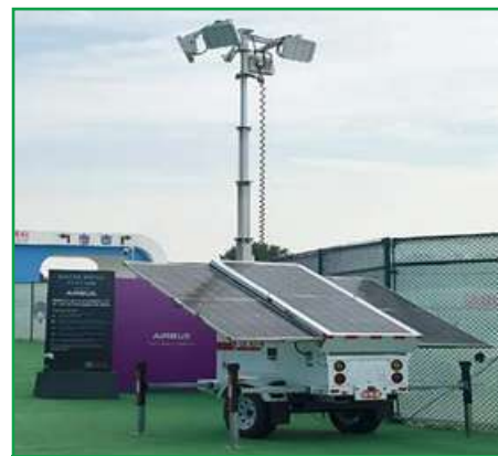
Solar-powered Lighting Towers
