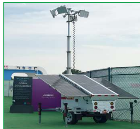
Solar-powered Lighting Towers
