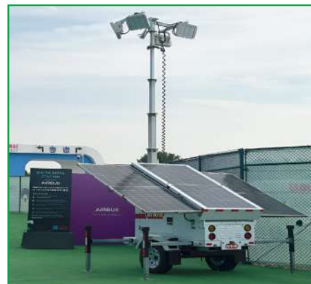
Solar-powered Lighting Towers
